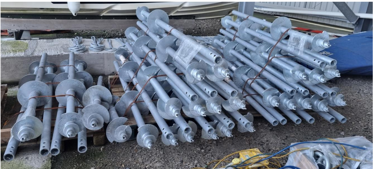
Photo: Screw anchors ready to install with Hazelett moorings in Studland bay (Studland Bay Marine Partnership)
